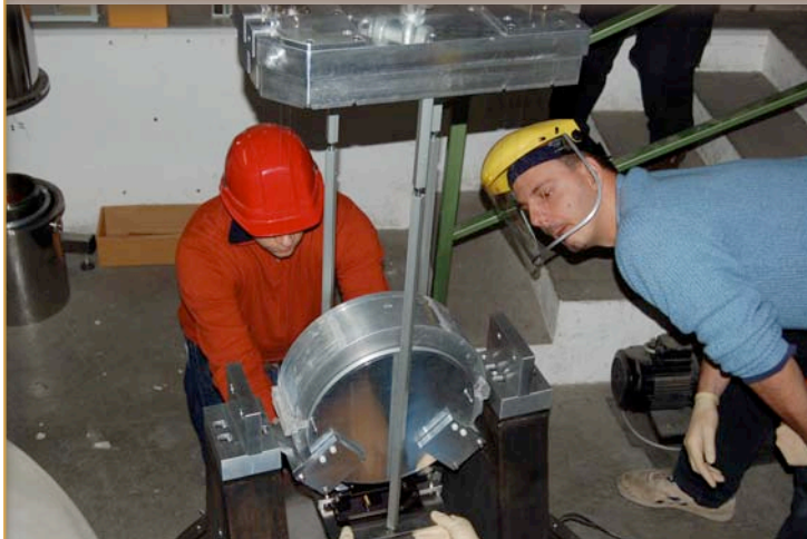
Dummy payload installation in the vacuum chamber
