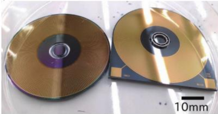
Figure 4. MEMS rotational electret energy harvester. A ball bearing is successfully installed its housing etched into the Si substrate. a) Rotor and stator substrate with a ball bearing, b) Rotational energy harvester stored in a plastic package.
